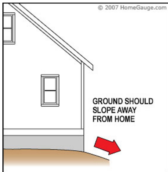
2.9 Item 1(Picture) Drainage Diagram
