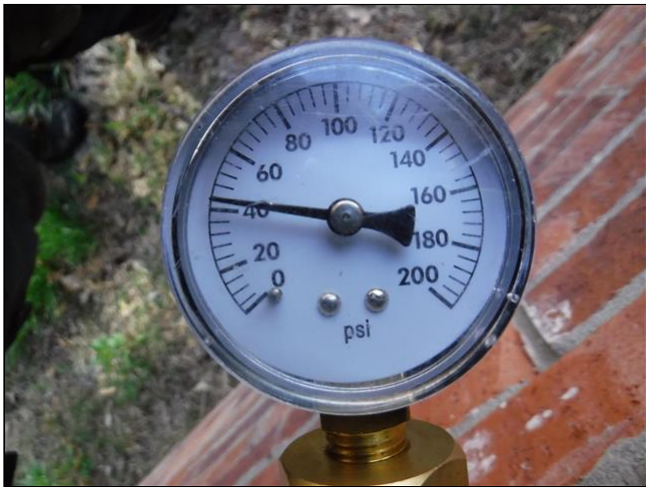
~42psi Water Pressure (60-80psi recommended)
